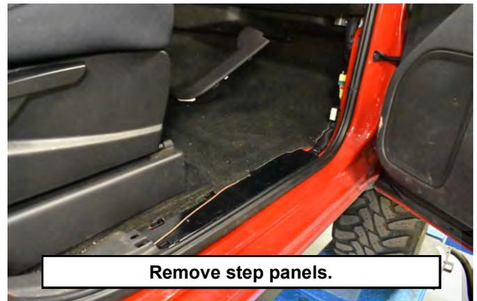
13. Remove the front kick panels by pulling up and away from the floor. **Photo 13**
